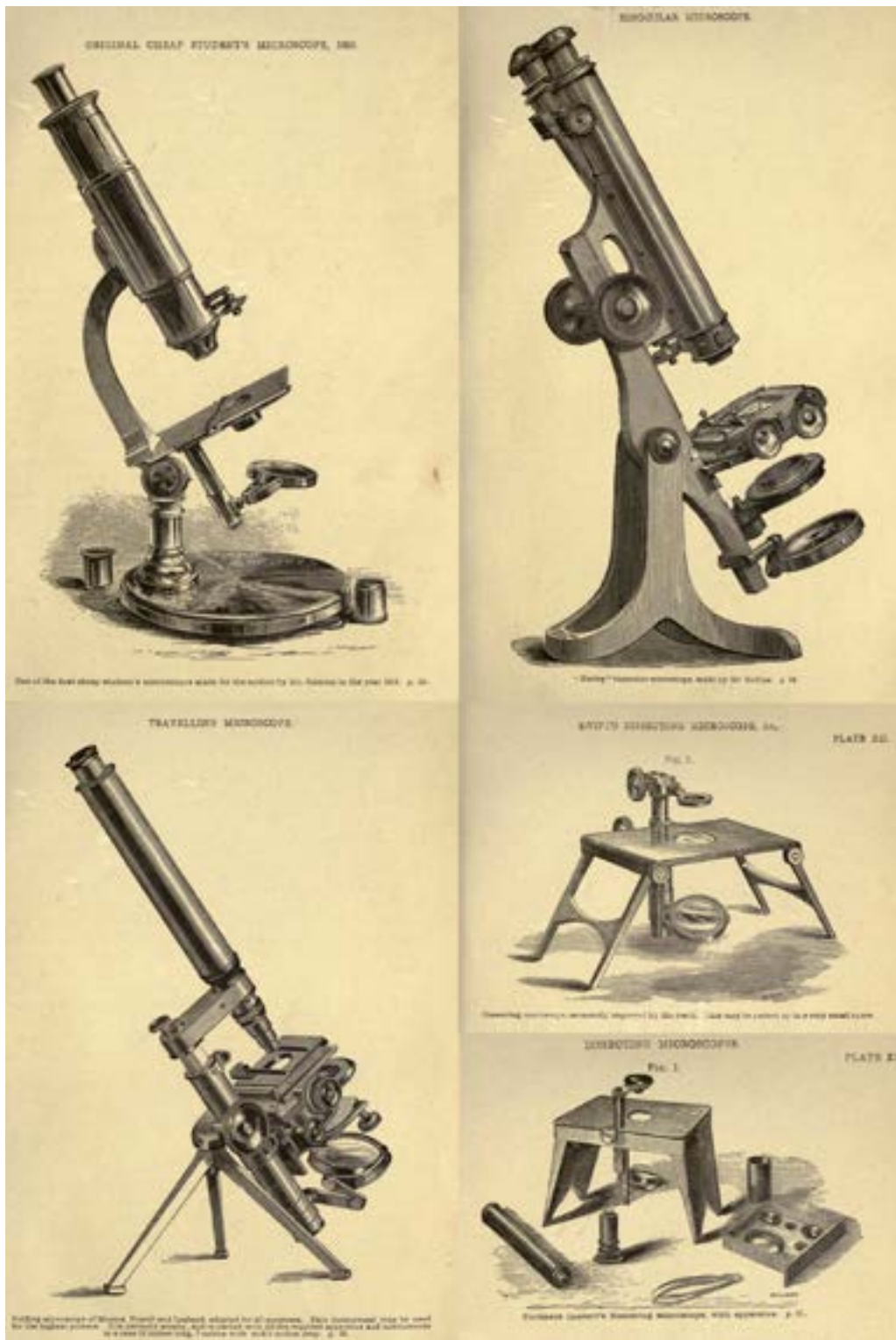
Figure 109. Some microscopes of Endrés' times. Clockwise, the original cheap student's microscope (1853), the binocular microscope made by Mr. Collins, Swift's dissecting microscope, Professor Queckett's dissecting microscope (with accessories), and the traveling microscope of Messrs Powell and Lealand. From L.S. Beale, 1880. How to work with the microscope . Philadelphia, Lindsay and Blakiston.
