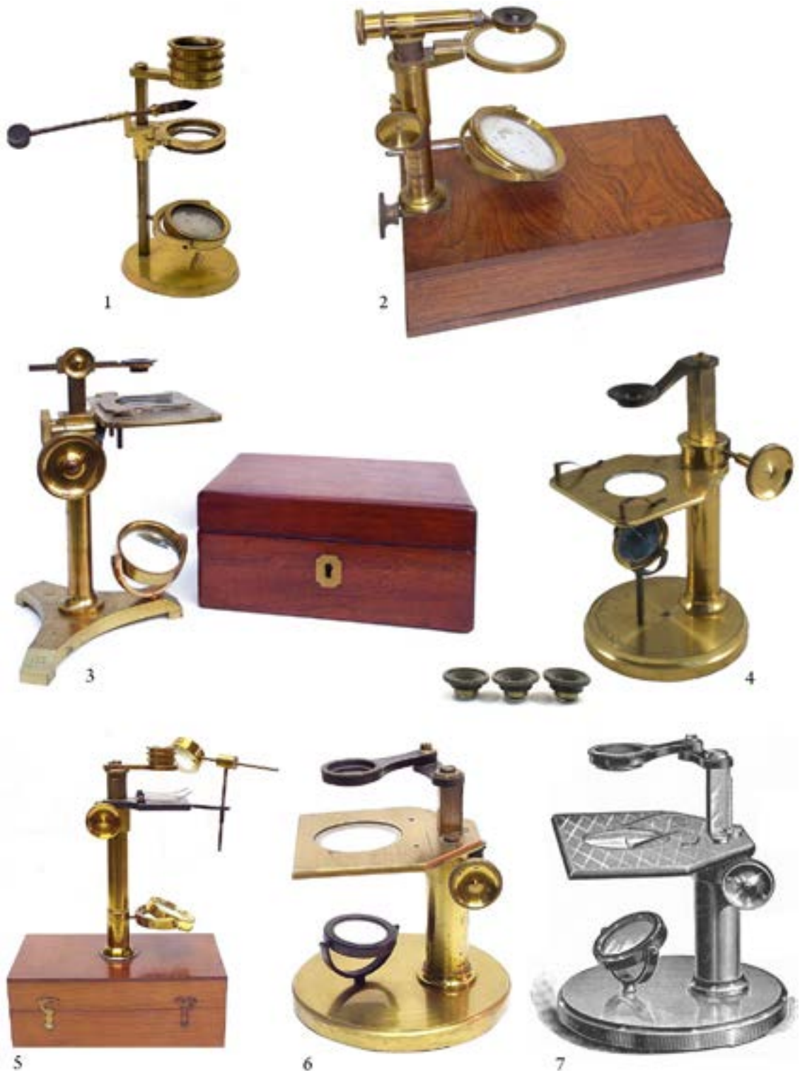
Figure 110. Botanical microscopes of Endrés' times. 1 – Dollond, London, ca. 1830. 2 – Deleuil simple microscope, Paris, 1835. 3 – A. Ross, London, 1850. 4 – Baker, dissecting simple microscope (with three magnification lenses), London, ca. 1860. 5 – J. W. Queen "Student's microscope", ca. 1870. 6 and 7 – J. Zentmeyer dissecting microscope, 1879.
